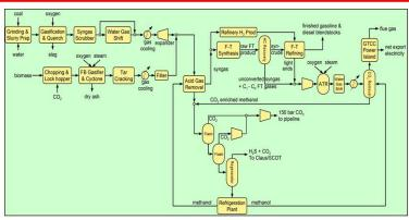
This FTL system [based on Liu et al. (2011)] was designed to make diesel + gasoline + electricity with CCS from coal and biomass (switchgrass) via slurry-phase F-T synthesis (iron catalyst) in a once-through synthesis reactor. Process starts with gasification: GEE entrained flow gasifier for Illinois # 6 coal + separate GTI fluidized bed gasifier for switchgrass.
